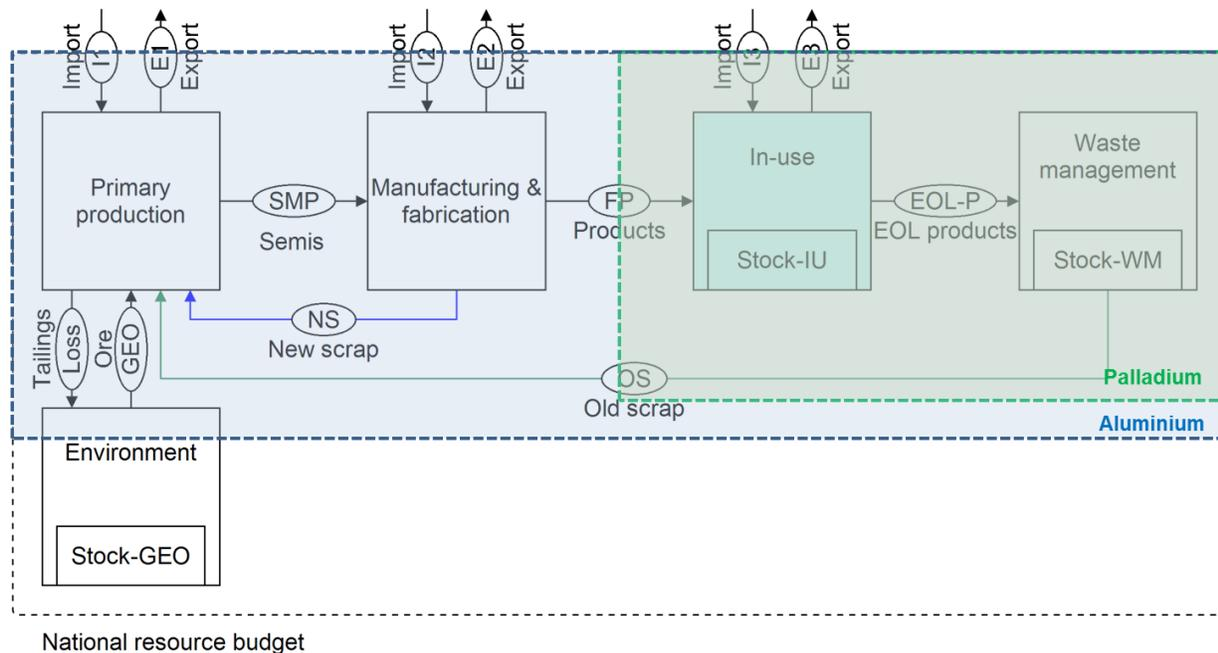
**Figure 2** Generic national material flow model indicating the scope of the case studies: Al use in Austria (blue shaded area) was investigated along the whole lifecycle (there is no (longer) bauxite mining in Austria). Pd flows in Austria were determined with a focus on flows in consumer products and wastes (green shaded area).
