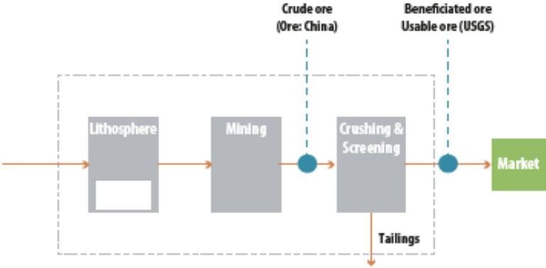
Figure 2: An illustration of the measurement points for crude and beneficiated ore
