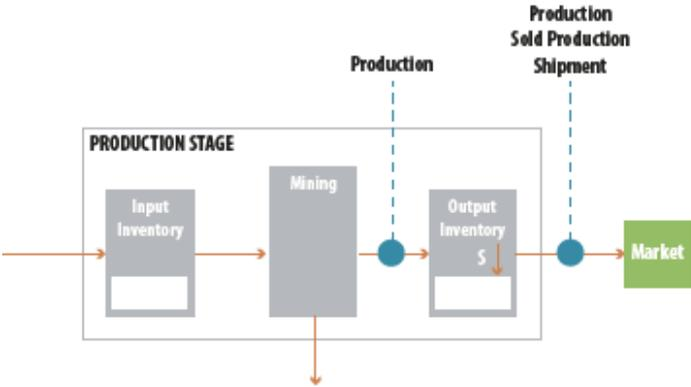
Figure 3: An illustration of the measurement points for production and production sold / shipment
